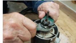
Image 3 shows the spanner configuration for tightening the collet. Spanner 'A' is on the bottom fixed spindle nut (obscured by the spanner and the centre 'floating nut') and spanner 'C' is on the top collet nut.
