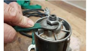
Image 2 shows the 'new floating nut' that has been missing for a long time. This nut is held with spanner 'B' when unlocking the collet nut and only when unlocking; it is not used when locking.
