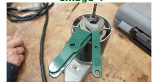
To loosen the collet, spanners 'A' and 'B' are held together and spanner 'C' rotated anti clockwise.
